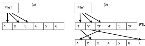
**Figure 1: File1 is using blocks 1, 2, and 3 on the drive. (a) In the case of the hard drive, these blocks are generally used directly. (b) In an SSD, the FTL masks the real arrangement of data and hides the behaviour of the drive.**
